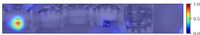
Figure 8: Heat map visualization of the relative importance of each pixel in the visual input of the drone towards its velocity command. Red regions have the most influence on the control command, whereas blue regions contribute the least. Best viewed in color.
