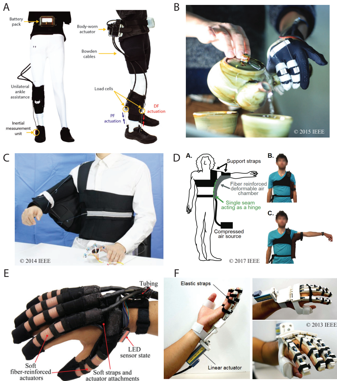
Figure 2 – Examples of wearable devices. A) Cable-driven lower limb exoskeleton [17]. B) Cable-driven hand exoskeleton [18]. C) Cable-driven upper body exoskeleton [19]. D) Pneumatic upper body exoskeleton [20]. E) Pneumatic hand exoskeleton [21]. F) Slide spring mechanism for hand exoskeleton [22].
