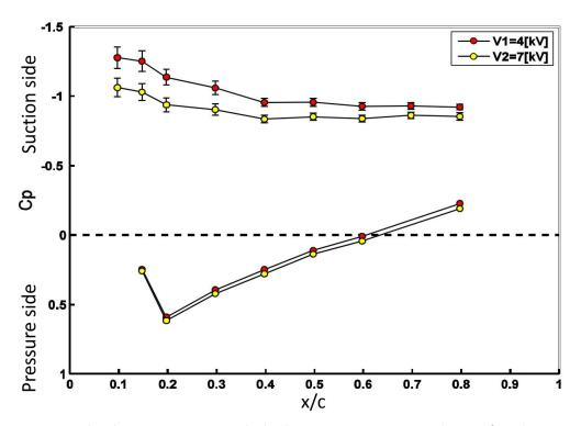
**Figure 23.**  $C_p$  distribution comparing applied voltages at Re = 200,000 and  $\alpha = 16^{\circ}$ , and actuation frequency f = 266.6 Hz.
