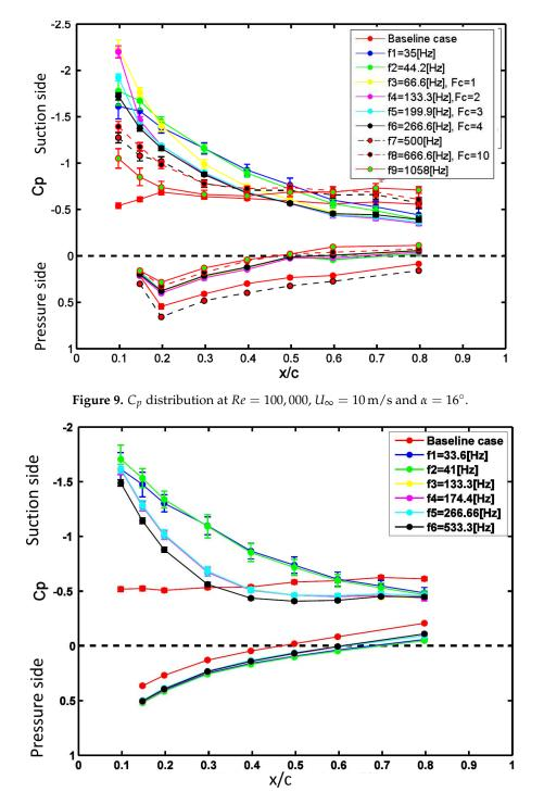
**Figure 10.**  $C_p$  distribution at Re = 200,000,  $U_{\infty} = 20$  m/s and  $\alpha = 16^{\circ}$ .
