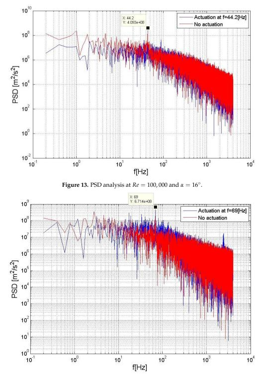
**Figure 14.** PSD analysis at Re = 200,000 and  $\alpha = 24^{\circ}$ .
