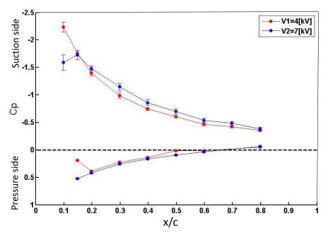
**Figure 18.**  $C_p$  distribution comparing applied voltages at Re = 100,000 and  $\alpha = 16^{\circ}$ , and actuation frequency f = 66.6 Hz.
