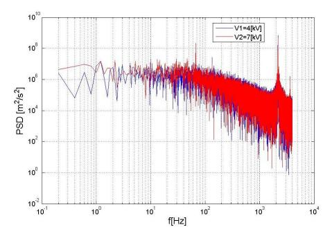
**Figure 19.** PSD analysis comparing applied voltages at Re = 100,000 and  $\alpha = 16^{\circ}$ , and actuation frequency f = 66.6 Hz.
