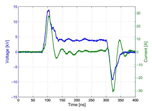
Figure 4. Sample current and voltage waveforms for the ns-pulse (NS-P) power supply.
