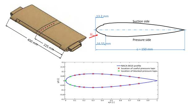
**Figure 1.** (top) A 3D view of the model used with a NACA 0015 profile (top left) with the insert indents for fixing to the Wind Tunnel section side walls, and a cross-section of the model showing the recess in the profile. (bottom) The profile "blown-up" in the y-direction for clarity to see the marked pressure tap locations used. The green ones were blocked by the actuator.
