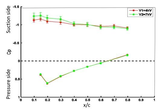
**Figure 22.**  $C_p$  distribution comparing applied voltages at Re = 100,000 and  $\alpha = 16^{\circ}$ , and actuation frequency f = 66.6 Hz.
