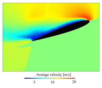
**Figure 26.** Velocity field at Re = 100,000 and  $\alpha = 16^{\circ}$  and DBD actuation at  $F_c^+ = 1$ .
