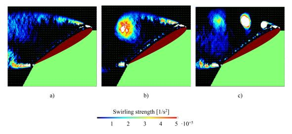
**Figure 27.** Swirling strengths at Re = 200,000 and  $\alpha = 24^{\circ}$ : with no actuation (**a**); at actuation frequency of 69 Hz, (**b**); and at actuation frequency of 266.6 Hz, (**c**).
