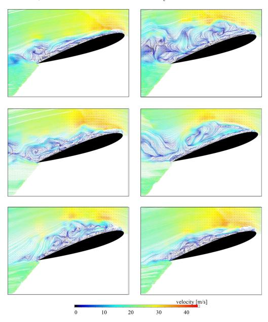
**Figure 24.** Evolution of different instantaneous flow structures and vortices with plasma actuation at  $F_c^+ = 1$  and Re = 100,000 (constant flow conditions).
