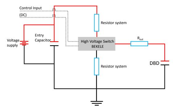
**Figure 3.** The ns-pulse (NS-P) power supply setup, developed in-house at EPFL by the Swiss Plasma Centre.
