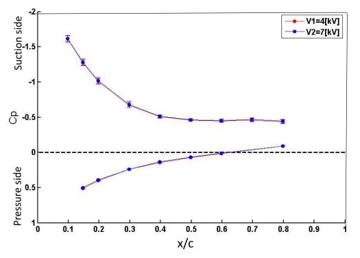
**Figure 20.**  $C_p$  distribution comparing applied voltages at Re = 200,000 and  $\alpha = 16^{\circ}$ , and actuation frequency f = 174.4 Hz.
