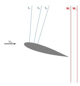
**Figure 5.** Location of measurement lines used to obtain the power spectra of flow instabilities without actuation.
