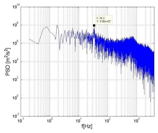
**Figure 7.** Power spectra along L1, Re = 100,000 and  $\alpha = 24^{\circ}$ .
