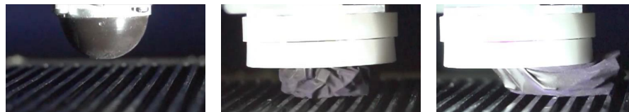
Figure 4.10 – Images extracted from high-speed recordings. Left: OF at 80 ms after touchdown in rebound; Middle: JMSS at 80 ms in hardened state without rebound; Right: JMA at 1.5 s with stretched membrane in steady-state sliding motion.
