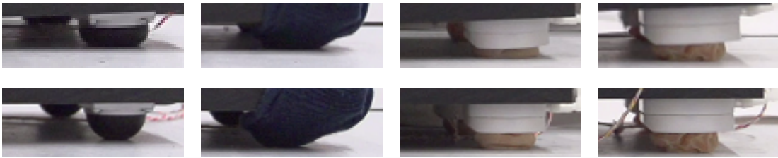
Figure 4.6 – Snapshots of the damping tests. The first row shows the elastic and plastic deformation of one foot during the first compression after releasing the platform from 5 cm. The second row shows the plastic deformation of the same foot after the platform comes to a rest. 1. column - OF, 2. column - OFS, 3. column - JMA, 4. column - JMV
