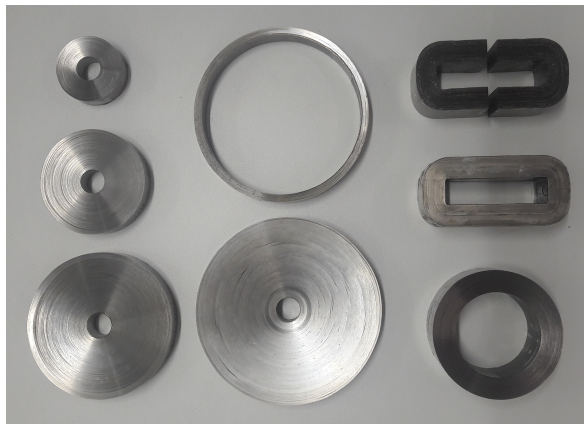
Fig. 5.25 Custom made core samples for experimental verification. First two columns: toroidal core samples that cover a wide A/R_m geometry range. Last column: cut and uncut U cores with identical size and their equivalent toroidal core.
