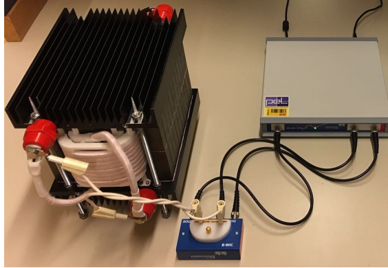
Fig. 7.2 Measurement of the electric parameters of the MFT
