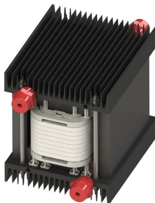
Fig. 6.5 A 3D render of the optimal MFT design, generated and selected according to the described design optimization procedure.
