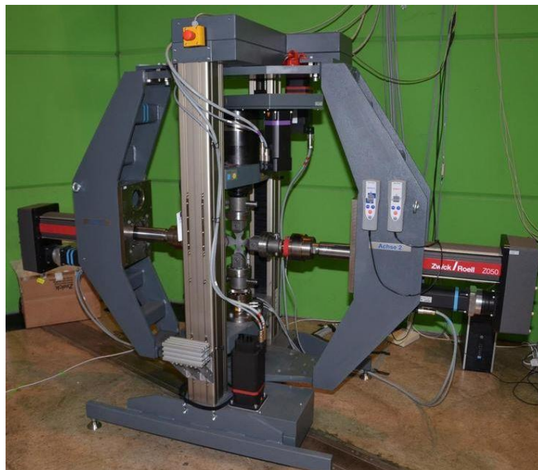
Figure 2-10 Large-scale multi-axial deformation rig at POLDI beamline (SINQ, Paul Scherrer Institute).
