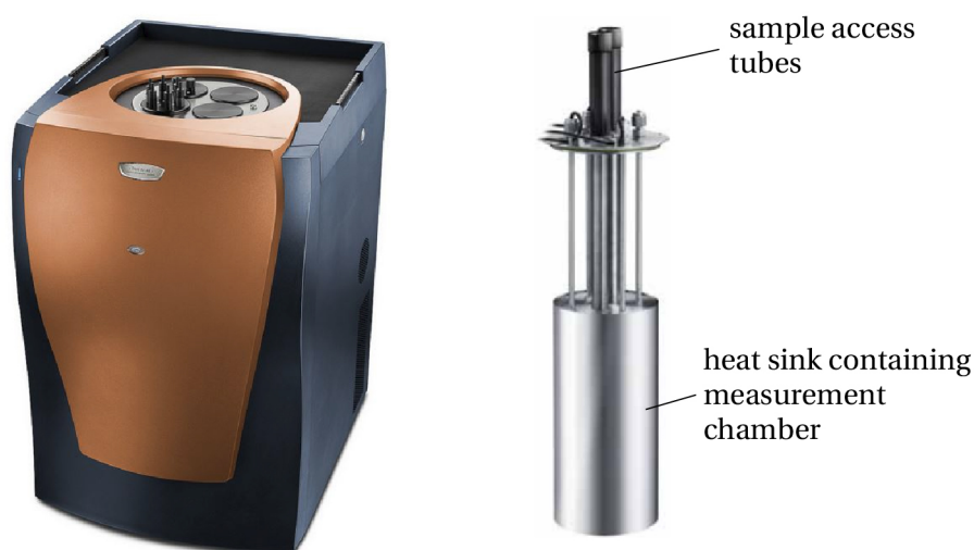
Figure 2.1 – Commercial IMC device for heat flow measurements. The TAM IV series (TA Instruments, USA) offers mL-sized ampoule-based calorimetric measurements, with possibility to perform up to 48 measurements in parallel. The sample ampoules are embedded in a massive thermostat. The injection of compounds, e.g. for the determination of mixing enthalpies or the quantification of binding energies is possible in open ampoule configurations. Reproduced from [65].
