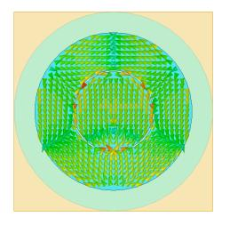
Fig. 3: Current distribution of antenna at 2.45GHz.
