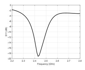
Fig. 4: Reflection coefficient
