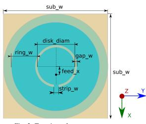
Fig. 2: Top view of antenna geometry.
