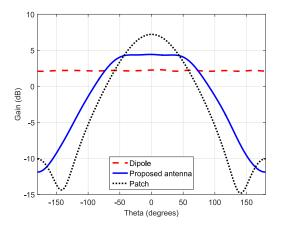
Fig. 7: Comparison of YZ pattern cut at 2.45GHz for the three antennas.
