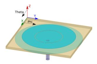
Fig. 1: Antenna 3D geometry.
