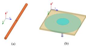
Fig. 6: Canonical dipole (a) and patch (b).
