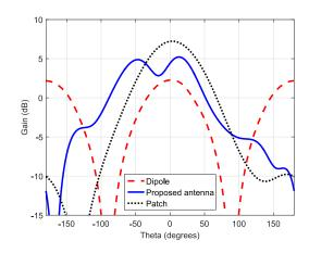
Fig. 8: Comparison of XZ pattern cut at 2.45GHz for the three antennas.
