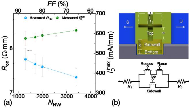
Fig. 5. (a)  $R_{ON}$  and  $I_D^{\max}$  of the recessed tri-gate versus  $N_{NW}$  and  $FF$ . (b) Schematic and equivalent circuit of the recessed tri-gate region.
