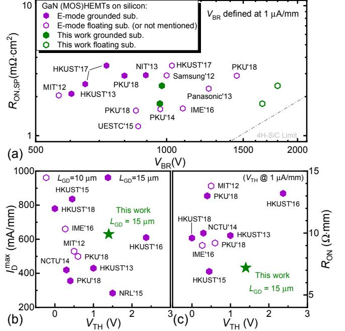
Fig. 7. Benchmarking of (a)  $R_{ON,SP}$  versus  $V_{BR}$  of the recessed tri-gate against E-mode GaN-on-Si transistors, by defining  $V_{BR}$  at  $I_{OFF} < 1 \mu\text{A/mm}$  with floating and grounded substrates. (b)  $I_D^{\max}$  and (c)  $R_{ON}$  versus  $V_{TH}$  (defined at  $1 \mu\text{A/mm}$ ). For fair comparison,  $L_{GD}$  smaller than  $10 \mu\text{m}$ , and literature results with unspecified  $R_{ON,SP}$  or  $I_{OFF}$  were not included.
