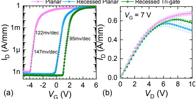
Fig. 2. Comparison of planar, recessed planar and recessed tri-gate devices. (a) Transfer at  $V_{DS} = 5$  V and (b) Output characters of the three device with  $V_G = 7$  V. The  $L_{GS}$ ,  $L_G$  and  $L_{GD}$  were 1.5, 2 and 15  $\mu\text{m}$ , respectively, and  $FF$  was 0.66.
