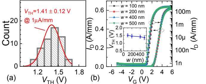
Fig. 4. (a) Distribution of  $V_{TH}$  of 56 recessed tri-gate devices. (b) Transfer characteristics of recessed tri-gate with different nanowire width. Inset: The extracted  $V_{TH}$  dependence with tri-gate nanowire width ( $w$ ).
