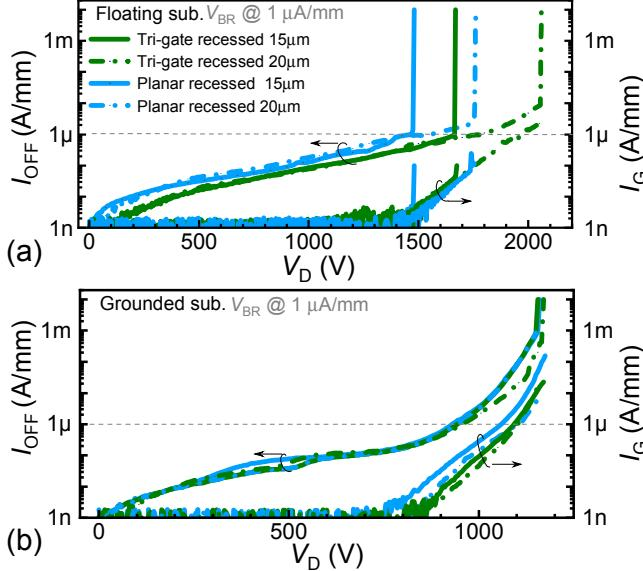
Fig. 6. Three terminal breakdown characteristics of recessed tri-gate ( $V_G = 0$  V) and recessed planar ( $V_G = -1$  V) MOSFETs with  $L_{GD} = 15 \mu\text{m}$  and  $20 \mu\text{m}$ , for (a) floating and (b) grounded substrate.
