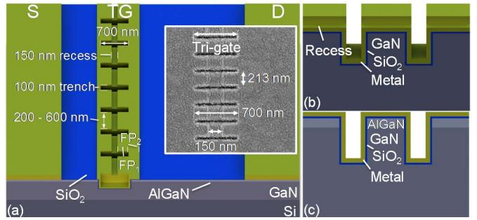
Fig. 1. (a) 3D schematic of recessed tri-gate MOSFET. Inset: zoomed SEM images of tri-gate regions. Cross-sectional views of recessed tri-gate MOSFET of (b) recessed regions and (c) tri-gate regions.
