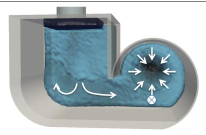
Figure 4: First part of the experiment, at low discharge there is no vortex, water leaves radially over the funnel crest, and the inflowing jet creates some counter flow towards the entrance. The head extraction position is given  $\otimes$
