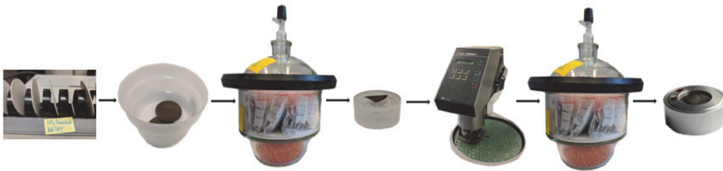
Figure 3-13. Sample preparation for SEM.
