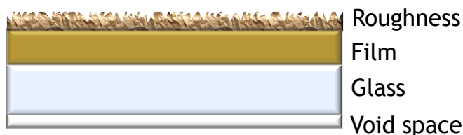
Fig. 8. Schematic of the global model used for bound multi-model fitting ellipsometry and transmission spectra of p -type \mu\text{c-Si:H} layers on glass.
