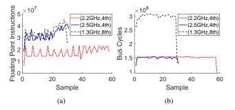
Fig. 1. Number of (a) floating point instructions and, (b) bus cycles, every 400 ms, under 3 system configurations: (frequency (GHz), number of threads)
