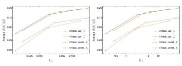
Normalized standard deviation of entry rates (after 10 min.) as function of  $\Gamma_m$  and  $\Pi_\beta$  for uniform and heterogeneous near-wellbore tortuosity.
