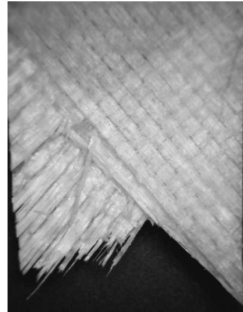
Fig. 3. Fatigue fracture surface.
