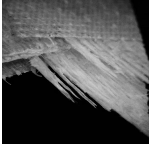
Fig. 7.2. Fatigue fracture surface of glass/epoxy composite with (\pm 45)_{2s} layout.
