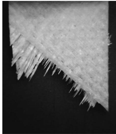
Fig. 2. Fatigue fracture surface.
