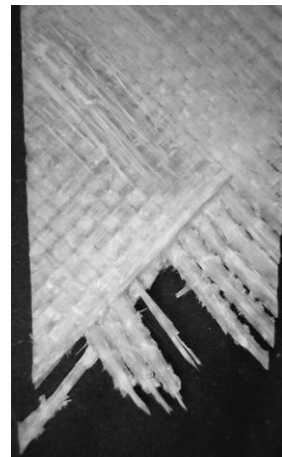
Fig. 3. Fatigue fracture surface.
