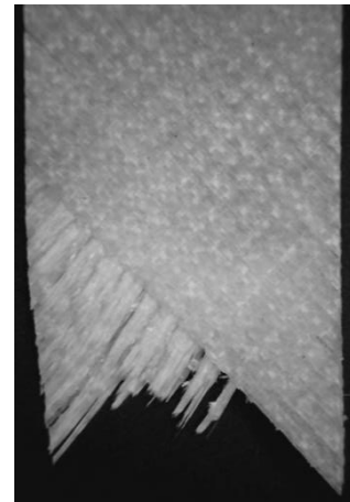
Fig. 3. Fatigue fracture surface.
