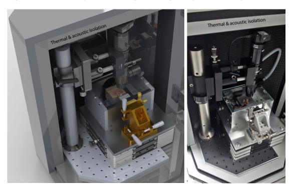
Figure 4.2 – New setup design contained in an enclosure for acoustic and thermal isolation (a) Rendering of the designed setup. The whole coupling setup, including imaging microscope, is contained in an acoustic enclosure. (b) Photo of the assembled setup.
