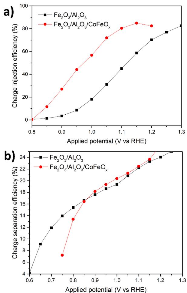
**Fig. 5** a) Charge injection efficiency showing an increased efficiency when CoFeO<sub>x</sub> is deposited and b) charge separation efficiency of blank hematite and CoFeO<sub>x</sub>-coated hematite.
