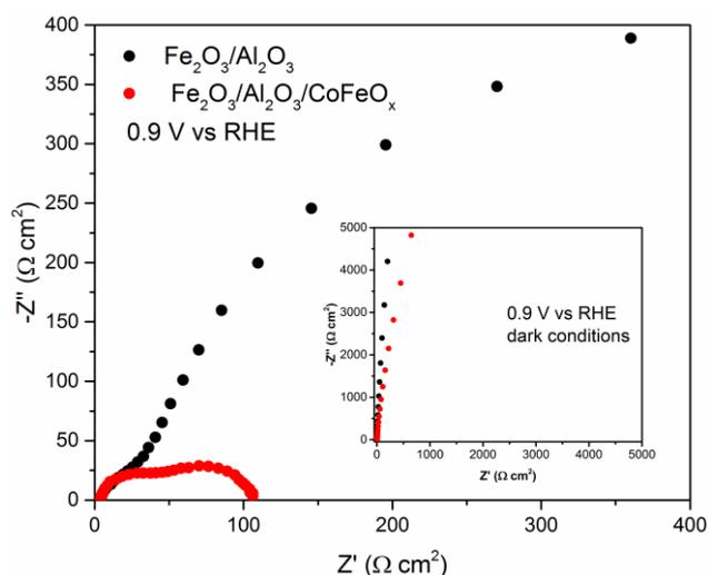
Fig. 6 Nyquist plot of Fe<sub>2</sub>O<sub>3</sub>/Al<sub>2</sub>O<sub>3</sub> and Fe<sub>2</sub>O<sub>3</sub>/Al<sub>2</sub>O<sub>3</sub>/CoFeO<sub>x</sub> at 0.9 V vs RHE in 1 M KOH and under illumination and in the dark (inset).
