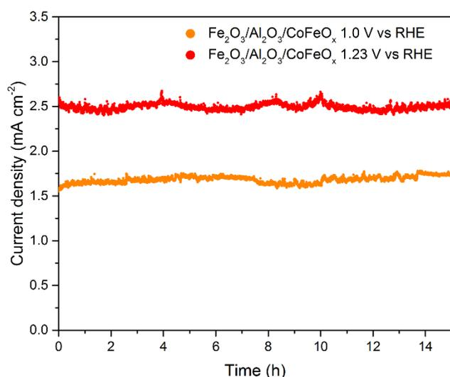
**Fig. 2** Constant potential photoelectrolysis at 1.0 and 1.23 V vs RHE of the CoFeO<sub>x</sub>-coated hematite during 15 hours under AM1.5 illumination in 1 M KOH.
