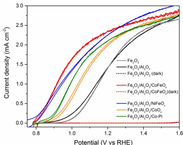
Fig. 1 Polarization curves in 1 M KOH of Fe<sub>2</sub>O<sub>3</sub> and Fe<sub>2</sub>O<sub>3</sub> coated with Al<sub>2</sub>O<sub>3</sub> and different OER catalysts under simulated AM1.5 illumination (lines) and in the dark (dots). Scan rate 10 mV s<sup>-1</sup>
