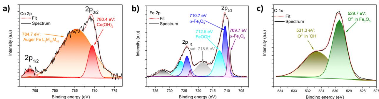
**Fig. 3** XPS spectra of the CoFeO<sub>x</sub>-coated hematite (5 LSV) with high-resolution spectra of a) Co 2p region, b) Fe 2p region and c) O 1s region, showing fits to spectra by deconvolution.
