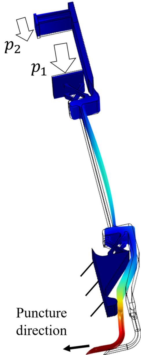
Fig. 13 Three-dimensional rendering of the deformation of the puncture mechanism based on finite element model (FEM) simulations
