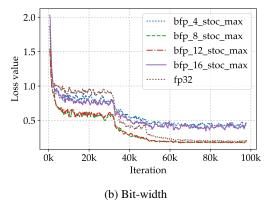
Figure 7. BFP design space exploration: training loss of ResNet-20 on CIFAR-10 with various BFP configurations.
