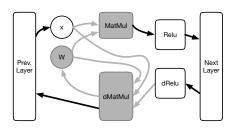
*Figure 3.* Traditional neural network layer dataflow using block floating point. The white boxes and black arrows indicate computations and values flowing in FP representation, and the grey boxes and arrows indicate operations and intermediate values in BFP.
