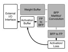
Figure 5. Hybrid BFP-FP accelerator with BFP
