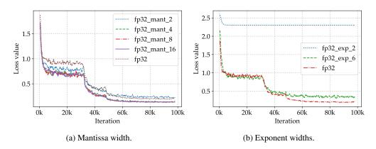
Figure 2. ResNet-20 training loss on CIFAR-10 with various floating-point configurations.
