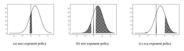
Figure 4. Matrix values rounded/saturated out by various exponent policies. The grey region of the curve indicates values that are lost when a tensor exponent is set. Values lost around 0 are rounded while other lost values are saturated.
