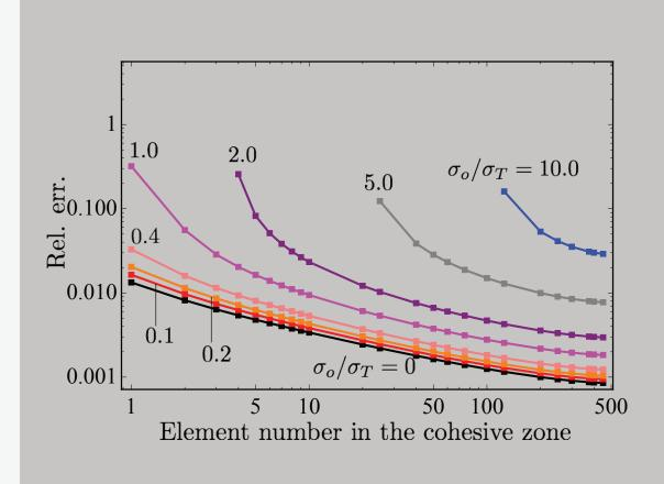
Mesh dependency of the stress accuracy ahead of the fracture tip (stress component of the element nearest to the fracture tip) for a uniformly-pressurized fracture with an impermeable cohesive zone.
