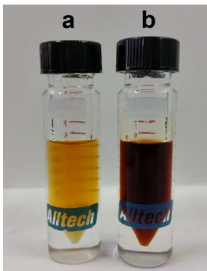
Figure 3.6 | Comparison of reaction mixtures after cellulose depolymerization. (a) Cellulose depolymerization with formaldehyde. (b) Cellulose depolymerization without formaldehyde. (Dark brown suggests a high degree of sugar degradation and humin formation).
