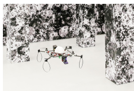
(e) LEQuad equipped with two fisheye cameras, it avoids collisions using optic flow computed across its 360 degrees field of view
