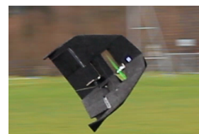
(f) YWing: a tailsitter VTOL capable of insect-like saccadic flight.
