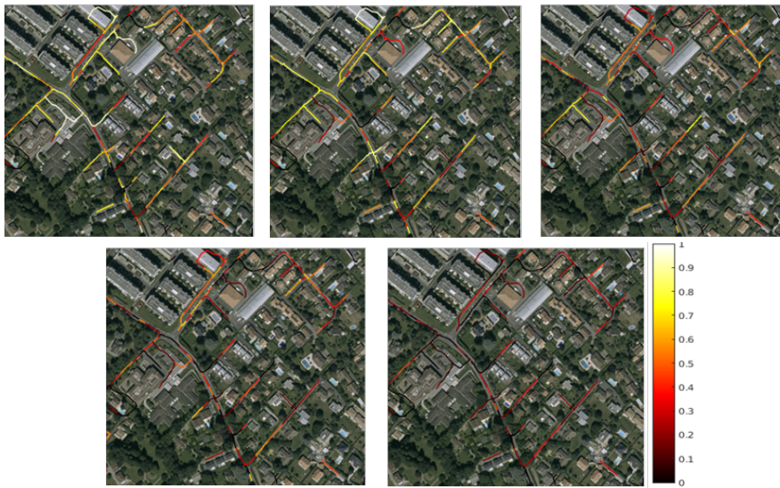
Figure 5.7 – Learning progress. Color-coded ambiguity of the training paths given by Eq. 5.9 after 5, 15, 25, 35 and 45 AL iterations. The measure was normalized across the iterations. There is a clear decrease in the uncertainty as the learning progresses.
