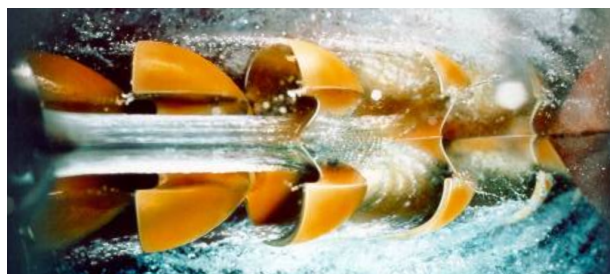
Figure 2.3 – Jet impingement on a reduced-scale Pelton runner [158].
