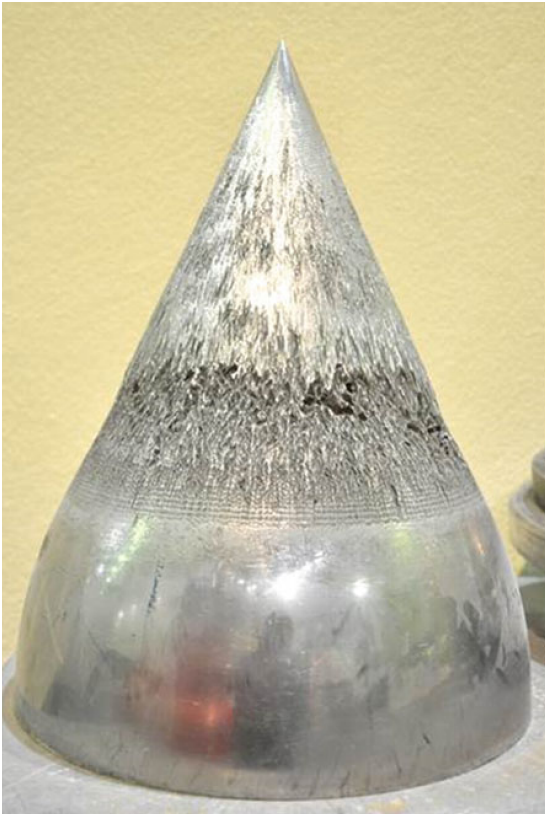
(a) Pelton injector needle after 165 operating hours under severe erosion conditions [203].
