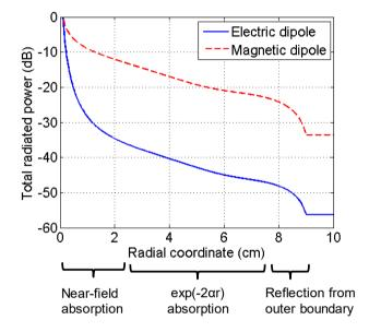
Fig. 1. Total radiated power as a function of the radial coordinate, for an elementary source implanted in the centre of a lossy host medium.
