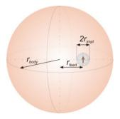
$r_{body} = 90 \text{ mm}$   $\varepsilon_{r,body} = 43.5 \text{-j} 34.75$  $r_{feed} = 0$
