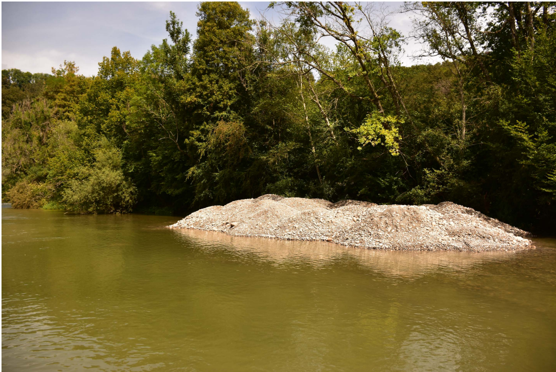
Figure 5.2 – Deposit I in the river before the flood experiment. Its dimensions correspond to about 22 m x 8 m x 1.5 m (length, width, height). The material was excavated from the adjacent riparian forest. Image courtesy Elena Battisacco.
