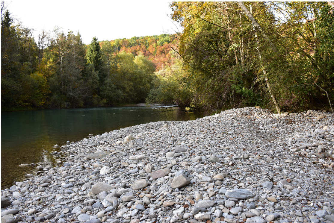
Figure 5.14 – View from deposit I towards upstream. An armoring of the residual deposit was observed. The armoring was sorted with large stones in the bottom (left), where the submergence was higher and cobbles (right) where the submergence was smaller. Image courtesy Severin Stähly
