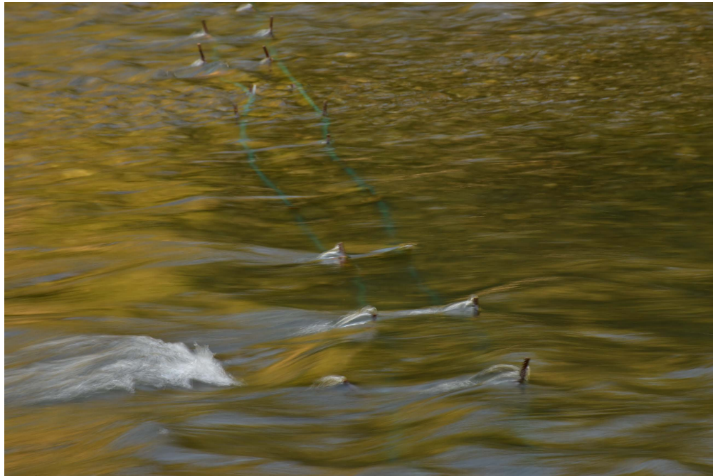
Figure 5.5 – Installed pass-over loop fixed-antenna in the Sarine river. The single loop cable was installed for protection inside a garden hose. The hose was fixed with cable straps to 1-m long vertical armoring irons installed in the river bed every meter. The antenna had a surface of 25 \times 0.3 \text{ m}^2 . Image courtesy Elena Battisacco
