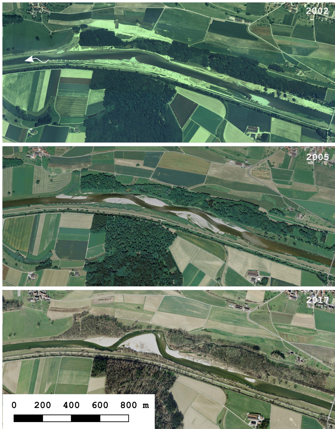
Figure 2.3 – Evolution of the Thur close to Altikon since its restoration in 2002. Image courtesy Swisstopo
