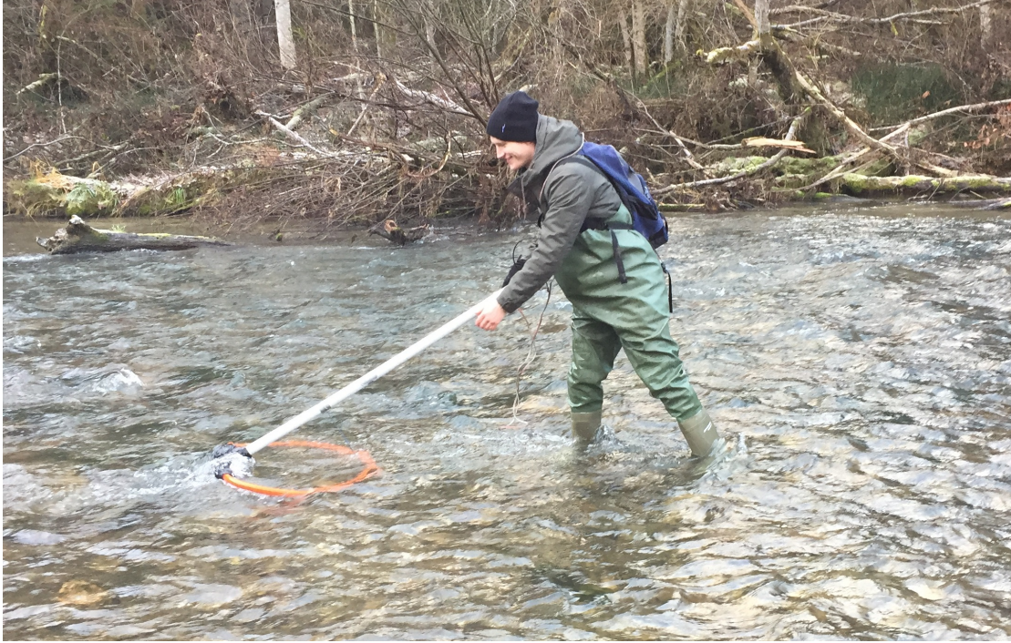
Figure 5.6 – Search of RFID PIT tags with the mobile antenna after the flood event in the Sarine river. Image courtesy Severin Stähly
