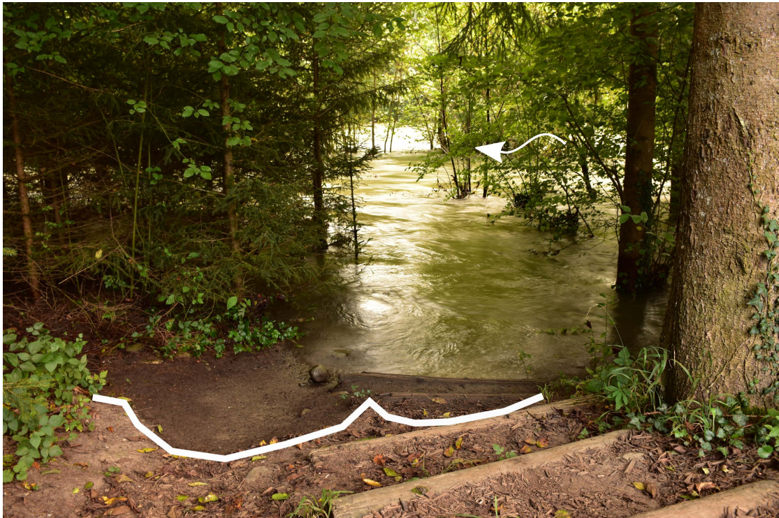
Figure D.6 – Water level in the Sarine 50 m downstream of deposit III after the peak discharge passed. The wetted boundary is marked with a white line and serves as a reference of the maximum water level. The elevation difference between the wetted area and the floodplain from where the photo was taken is more than 1 m. Flow direction from right to left. Image courtesy Elena Battisacco
