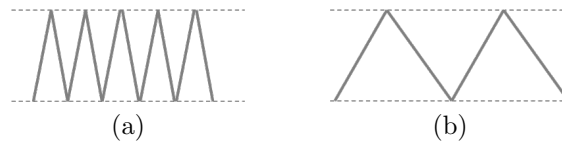
Figure 3.2: The two profiles (a) and (b) have the same R_a values.
