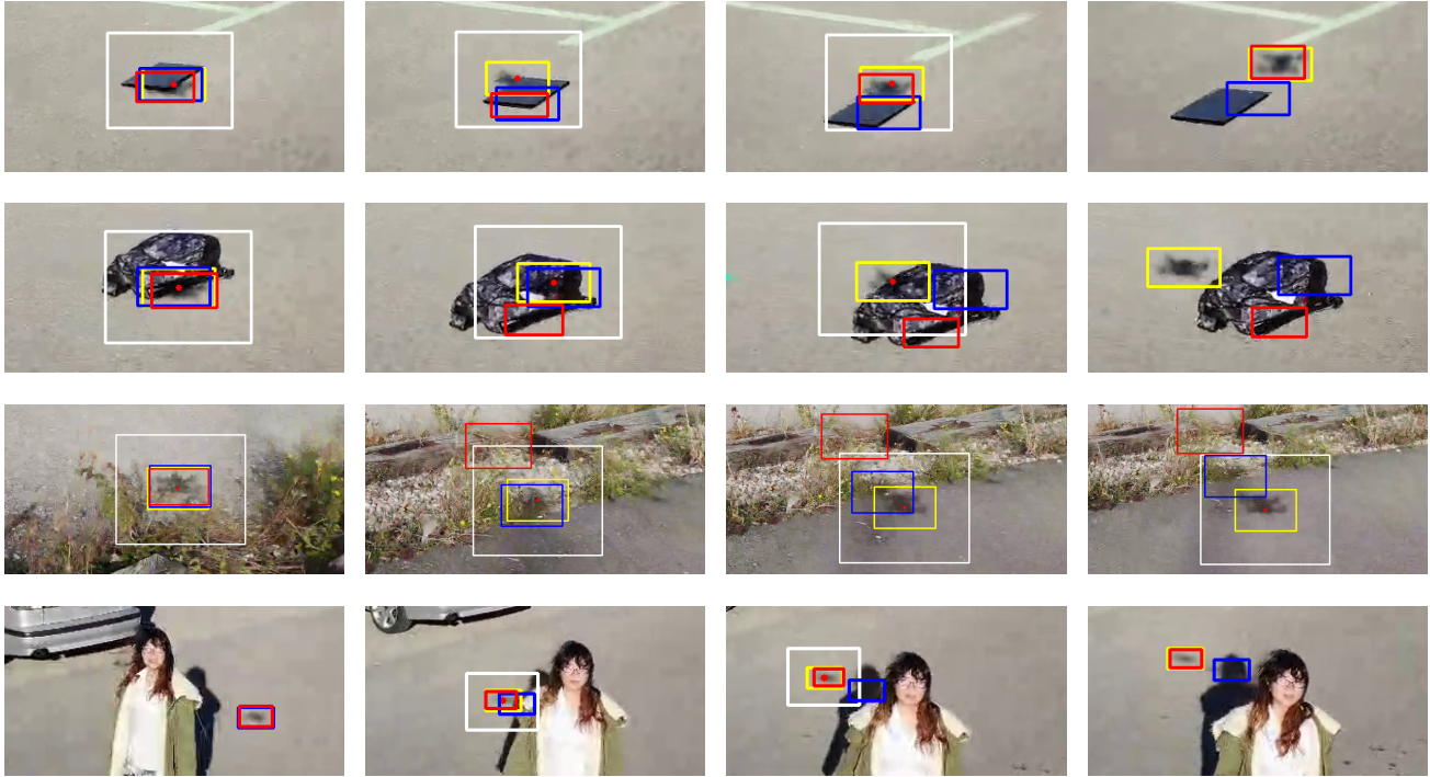
Fig. 4. Drone shadow tracking results on the 4 videos with difficult tracking scenes. Each row contains critical frames from one of the 4 videos (with time increasing from left to right). The blue box is the kernel-based tracking result of MOSSE [1], the red one is the deep learning based tracking result of DAT [9] and the yellow box is ours. The white box delimits S' .
