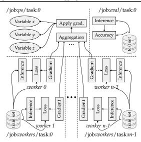
Figure 2. High-level components and execution graph. Each gray rectangle represents a group of tf.Operation, and each plain arrow represents a tf.Tensor. The sub-graph between the gradients to the variables corresponds to Equation 4. For readability purpose, the tensors from the variables to each "Inference" and "Gradient" groups of operations have not been represented.
