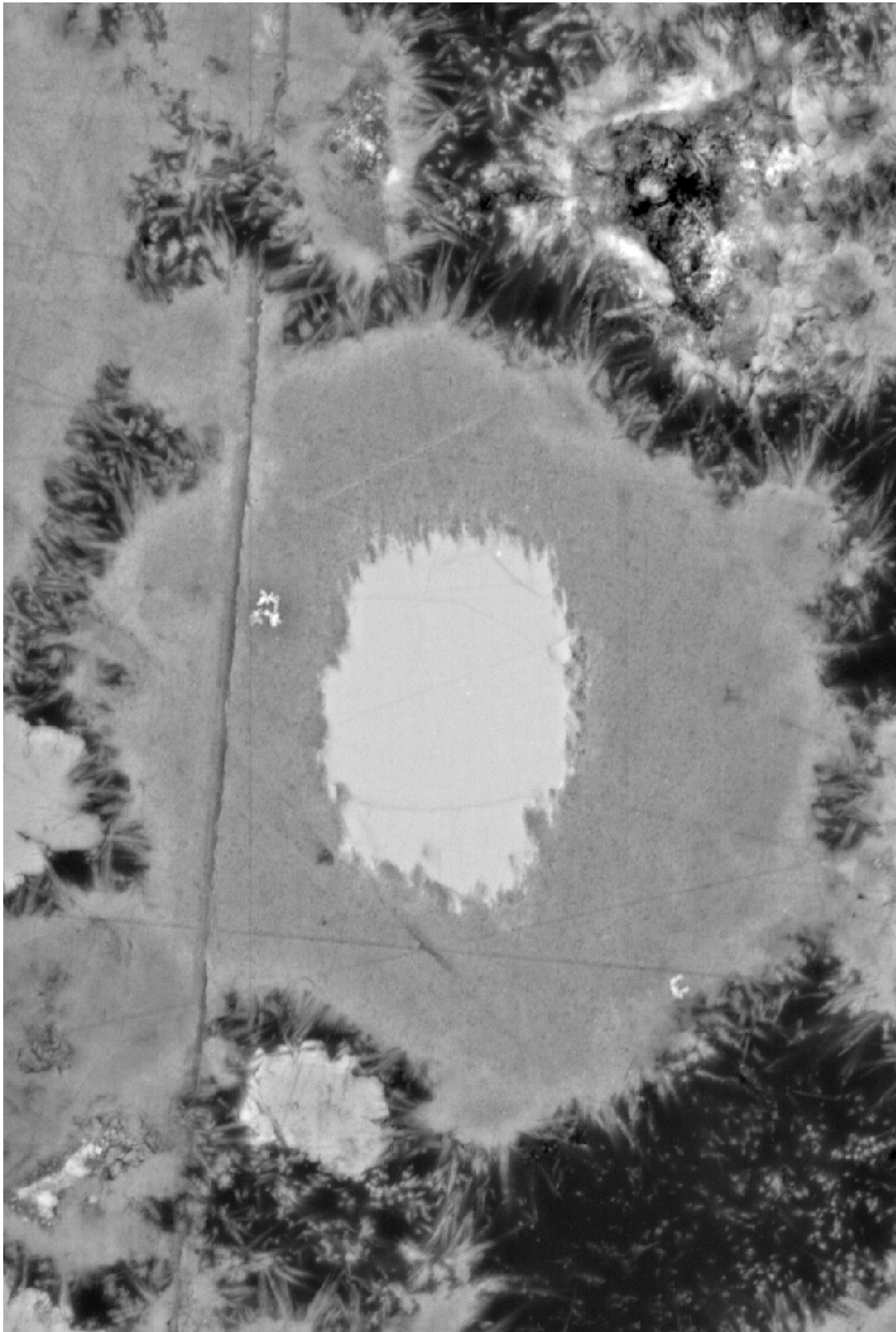
Figure 2.25 – SEM polished section of a w/c = 0.7 alite paste at 28 days. Sections of needles are observed (points) in many different areas, in particular in the bottom right. Etch pits are still plainly visible on the anhydrous core. The central grain largest diameter is 12\ \mu\text{m} , the vertical length of the image is 20\ \mu\text{m} . Image taken at 5 kV, working distance 6 mm. See the online version to get a better view of the needles sections.
