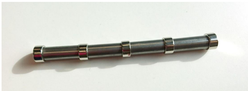
Figure 1. Photograph of the bar magnet that was built from five smaller disc magnets and separated by steel bars.
