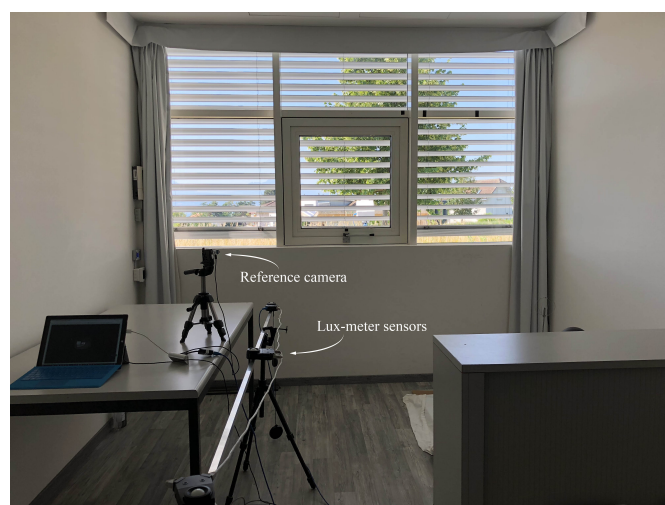
Fig. 5.8. Cross validation set-up with a reference camera
