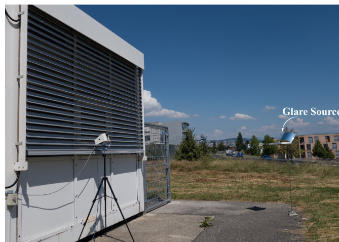
Fig. 5.18. Set-up of a curved mirror inserted manually as the glare source
