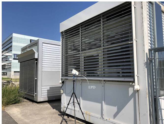
Fig. 5.2. Daylighting test module with automated 'Eye-sight' EVB
