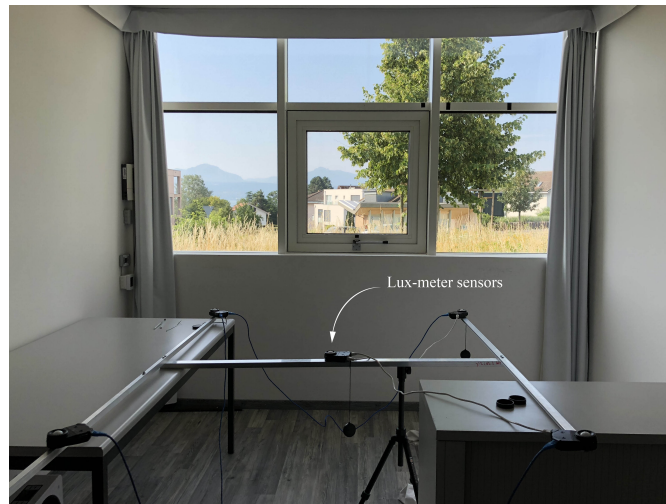
Fig. 5.12. Set-up of lux-meter sensors to monitor WPI as reference
