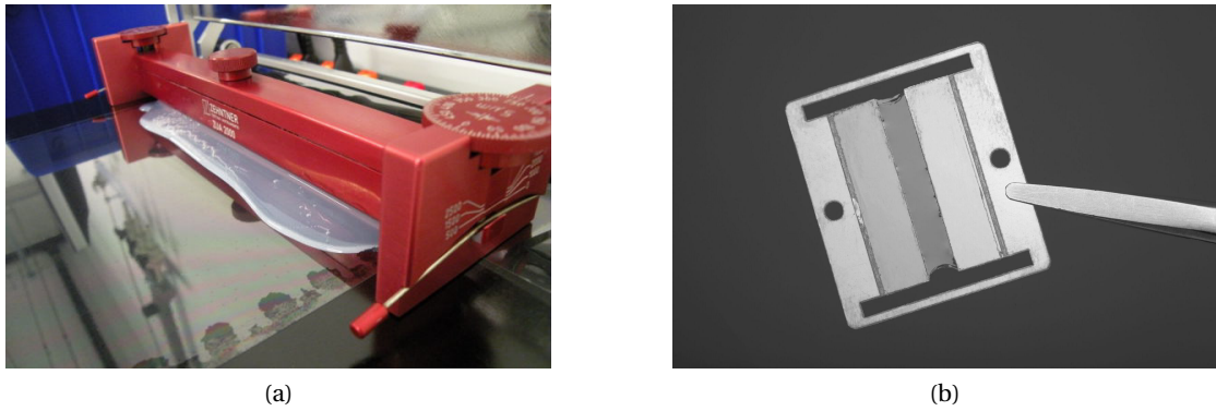
Figure 3.3 – (a) PDMS uncured solution is spread at the desired thickness on a PET foil using a blade coater. This method allow to have relative big area covered with PDMS [and high reproducibility of the membrane thickness. After curing in the oven, the membranes are suspended on PET frames as holders by water immersion. (b) Picture of a 1:6 aspect ratio suspended membrane.
