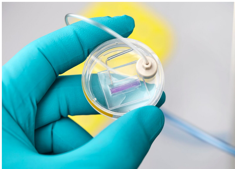
Figure 1.2 – Picture of the final device developed within this thesis and placed in a 55 mm diameter Petri-dish for cell culture.
