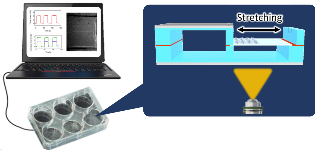
Figure 1.1 – Final working principle of the device developed within this thesis: the device allows simple acquisition of the measurement directly on the computer, its working principle is based on pneumatic actuation combined with a differential strain optical read-out.
