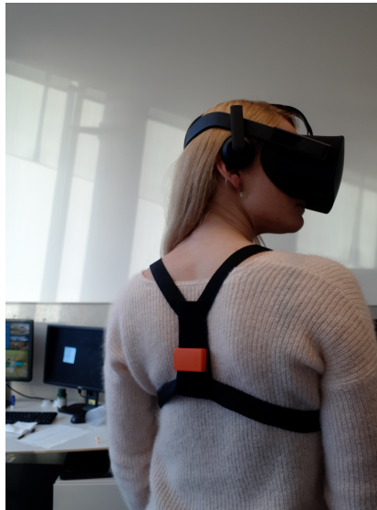
Figure 4.2 – Experimental setup including the Oculus Rift and one IMU placed in the back
