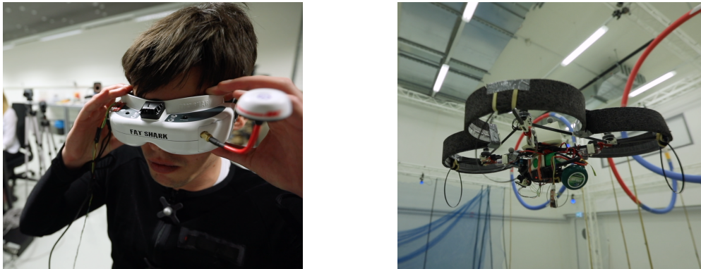
(a) Pilot wearing the HMD providing visual feed- (b) Custom-made quadcopter and circular gates to be crossed during the piloting task
