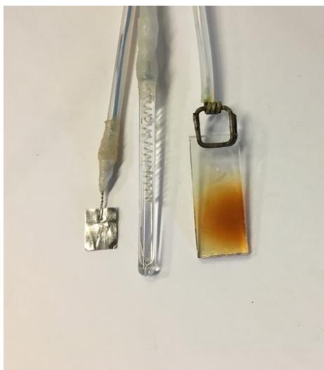
Supplementary Figure 1. Undivided cell for photoelectrochemical oxidation
