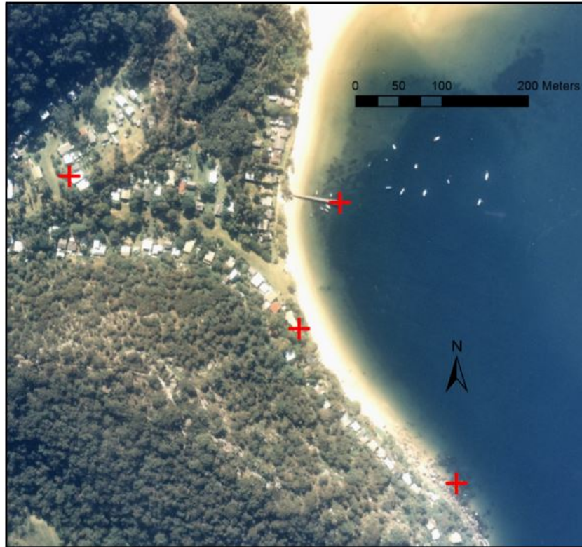
Figure 19: Example locations of ground control points used for the rectification of aerial photographs - Great Mackerel Beach
