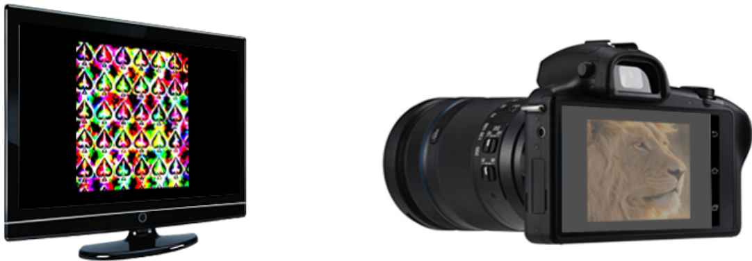
Figure 5.1 – A tempocode is a video (left) containing a hidden image that can be revealed through long-exposure photography of the video (right).
