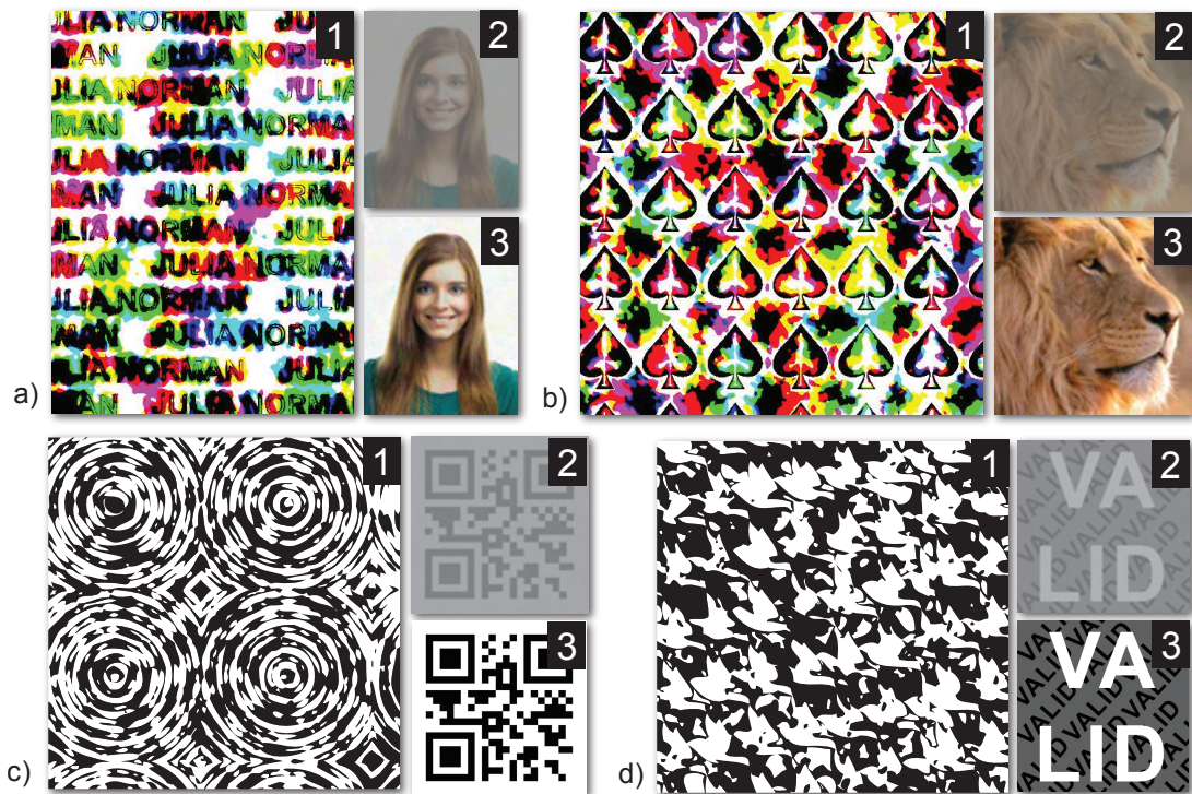
Figure 5.7 – Sample tempocode frames (1) generated with the different input images and the different dither matrices. The hidden images can be revealed by averaging (2). An inverse contrast-reduction operation yields the original input image (3). In all the cases, the target image is recovered by software averaging the original tempocode frames. We have the following parameters (a) for the woman, \alpha = 0.4 , (b) for the lion \alpha = 0.5 , (c) for the QR code \alpha = 0.2 , and (d) for the text, \alpha = 0.3 .
