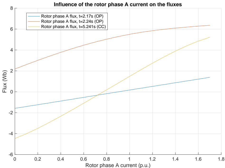
Figure 4.53 – Rotor flux of phase A as a function of the rotor current of phase A for different operating points (represented by CC=short-circuit and OP=nominal operation point). The results are shown for particular times only, which corresponds to maximal respectively minimal value of the inductance.
