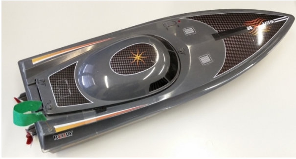
Fig. 3: An ASV, which can carry the surface beacons or serve as surrogates for the AUVs for various experiments.
