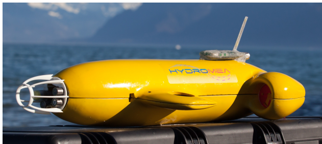
Fig. 1: The Vertex AUV with its sensor suite in the front, protected by a white cage. The AUV is about 70 cm long, weighs 7 kg, and can be carried and deployed easily by one person.
