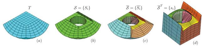
Figure 4: Untrimming and approximating trimming surfaces, S, in the parametric space of trivariate T. (a) The trivariate T in Euclidean space. (b) The trimming surfaces, S, also in Euclidean space. (c)  $\overline{S}$ , the untrimming of S in the Euclidean space. (d) Approximation of  $\overline{S}$  in the parametric space of T, by tensor product surfaces of orders 3x3.
