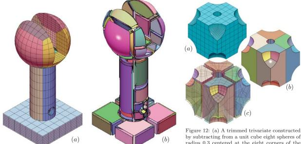
Figure 11: Untrimming of a V-model. (a) The V-model consisting of 20 trimmed trivariates. (b) The result of untrimming each of the trimmed trivariates of the model, resulting in 370 tensor product B-spline trivariates displayed in an exploded view.
