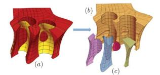
Figure 2: Subdivision of trimmed trivariate (red) in (a) along an iso-parametric surface (yellow) results in five trimmed trivariates: one trimmed trivariate on the back side of the iso-surface in (b), and four trimmed trivariates on the front side of the iso-surface in (c). An exploded view is presented in (b)/(c).
