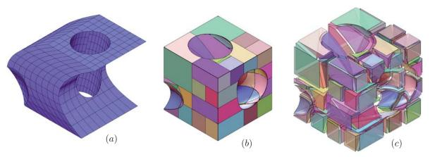
Figure 7: Untrimming of a trimmed Bézier trivariate. (a) A trimmed Bézier trivariate of orders (2,2,3). (b) Untrimming result in the parametric space of (a), yielding 262 tensor product B-spline trivariates shown in an exploded semi-transparent view in (c).
