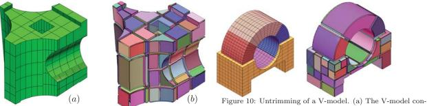
Figure 9: Untrimming of a trilinear trimmed B-spline trivariate with  $(4 \times 4 \times 3)$  Bézier domains. (a) The trimmed B-spline trilinear trivariate. (b) Untrimming of (a) yielding 406 tensor product B-spline trivariates displayed in an exploded view.
