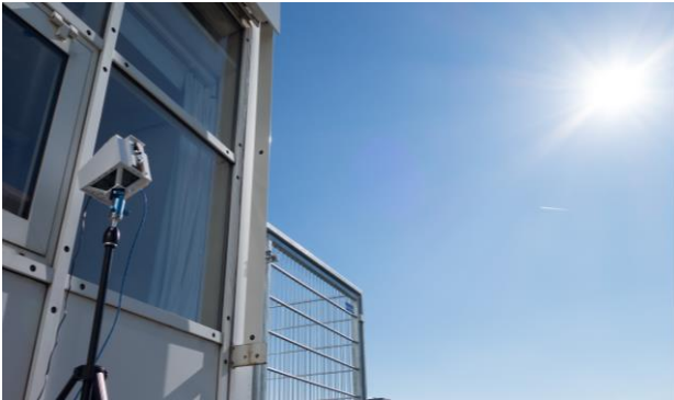
The embedded photometric device assessing work-plane illuminance based on sky monitoring.
