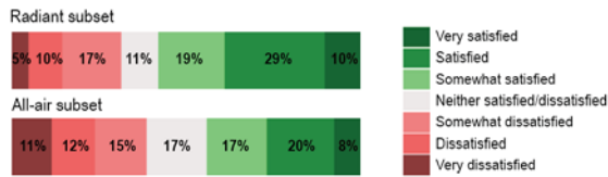
Figure 1: Bar chart showing the distribution of temperature satisfaction for the radiant and all-air subset
