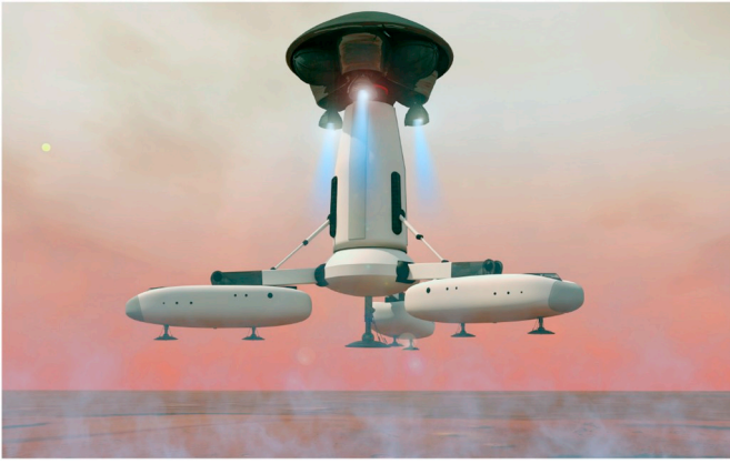
Fig. 18. Artist's view of the central core and the deployed capsules being deposited on Mars by the crane vehicle in the trade-off scenario.
