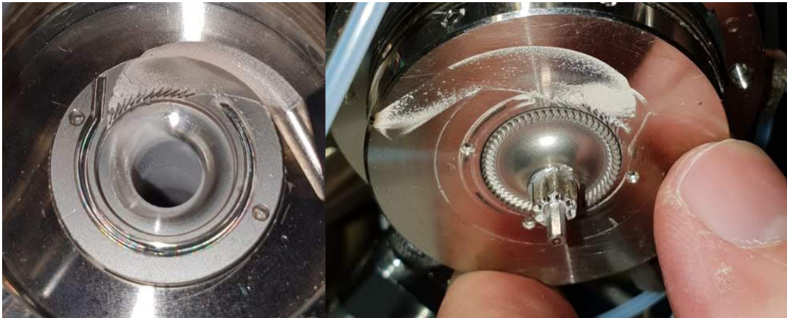
Figure E.1 – Turbine volute and stator (left), as well as turbine seal and rotor (right) with deposits: ceramics, salt, and glass fibers.
