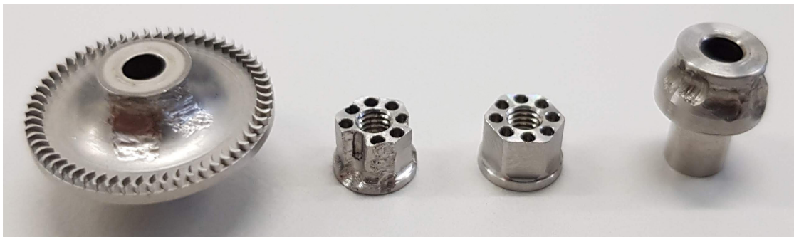
Figure D.1 – The radial inflow turbine with a diameter of 15 mm (left), the screw that fixes the turbine on the shaft with holes for balancing (middle) after several balancing procedures (second from the left) and before balancing (second from the right). A “dummy turbine” for removing the entire shaft during the balancing procedure is shown on the right.
