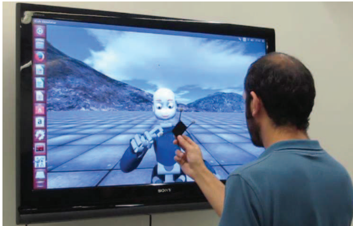
Figure 3.12 – The experimental setup. The avatar is displayed on a big screen (46 inches). The avatar led the mirror game and the participant followed the avatar’s hand motions. The participant held a marker for motion tracking purposes.
