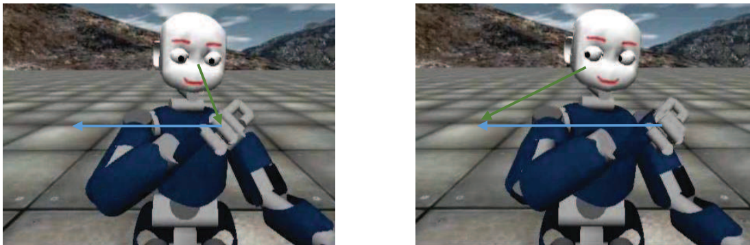
Figure 3.10 – The simulated iCub robot. The robot is acting as the leader in the mirror game, generating random sinusoidal trajectories. (Left) the gaze is fixated on the hand. (Right) the gaze precede the hand. The blue arrows show the next hand movement and the green arrows show the current gaze fixation point.
