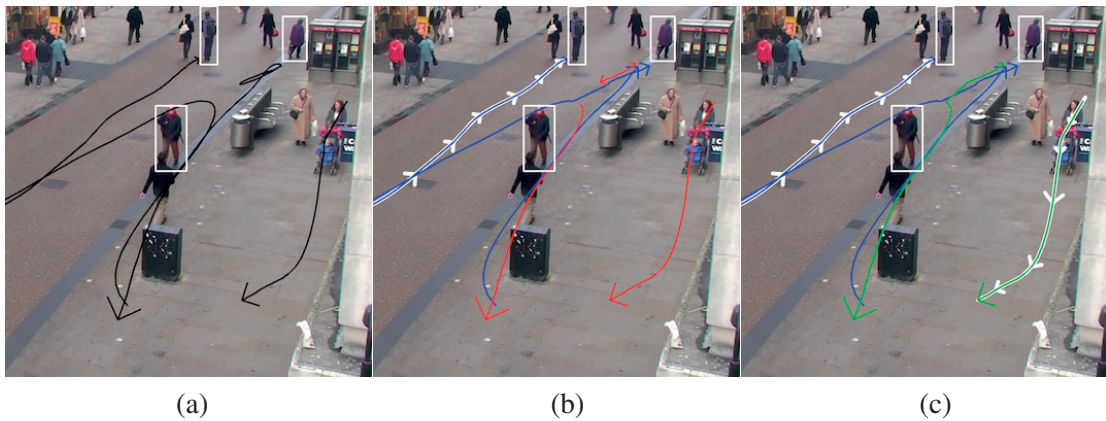
Figure 4.8 – Example of unsupervised optimization. (a) Four people are tracked using KSP . Trajectories are shown as solid black lines, bounding boxes are white. Tracks feature several identity switches. (b) First, alternating scheme finds a single pattern, in white, that explains as many trajectories as possible - that is the leftmost trajectory. Given this pattern, next step is the tracking. Trajectories in blue are the ones assigned to this pattern, trajectories in red are assigned to no pattern. One identity switch is fixed. (c) After several iterations, we look for the best two patterns. Rightmost trajectory is picked as the second pattern. Fitting trajectories to the best two patterns allows to fix the remaining fragmented trajectory. Trajectories assigned to the second pattern in green.
