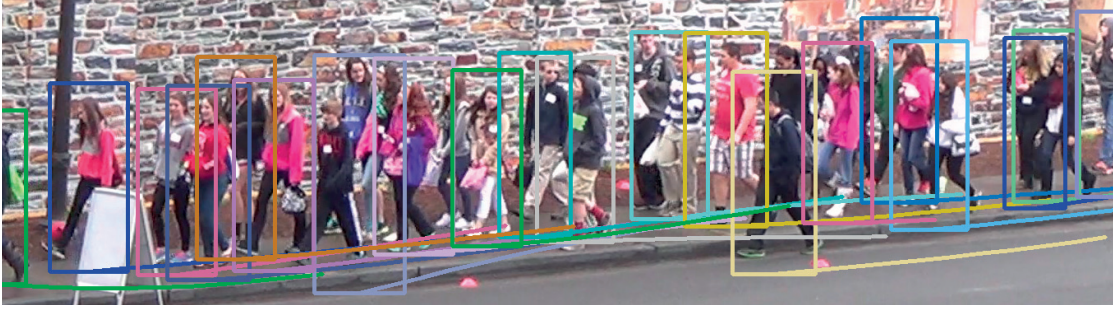
Figure 5.4 – Bounding boxes and the last 6 seconds of tracking, denoted by lines, in dense crowd on DukeMTMC dataset.
