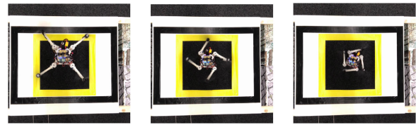
Fig. 6. Traversal of an horizontal gap using the O morphology. Left: the quadrotor approaches the gap with the X configuration (time t = 0 s). Center: the quadrotor starts the folding maneuver to adapt its morphology to the shape of the gap ( t = 1 s). Right: the gap has been traversed ( t = 2 s).
