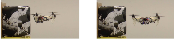
Fig. 7. Inspection of a surface using the T configuration (left) and the X configuration (right).
