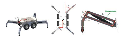
**Figure 1.** (**a**) front view of the mobile platform; (**b**) top view of the mobile platform; (**c**) scheme of a leg of the system.
