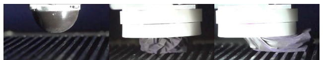
Figure 3: Snapshots from high-speed recordings. Left: OF at 80 ms after touchdown in rebound; Middle: GMSS at 80 ms in hardened state without rebound; Right: GMA at 1.5 s in steady-state sliding.
