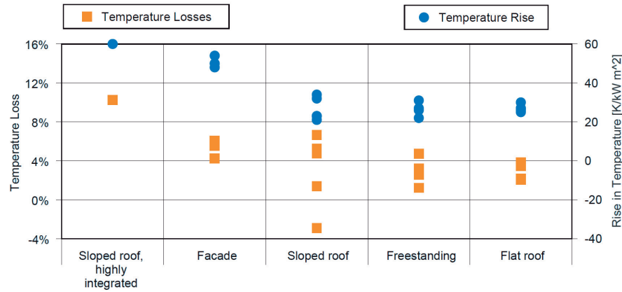
Figure 1.9 – Overview of temperature losses and the rise in module temperature of well-integrated sloped roofs, façades, well-ventilated roofs and freestanding and flat roofs (figure taken from [71]).
