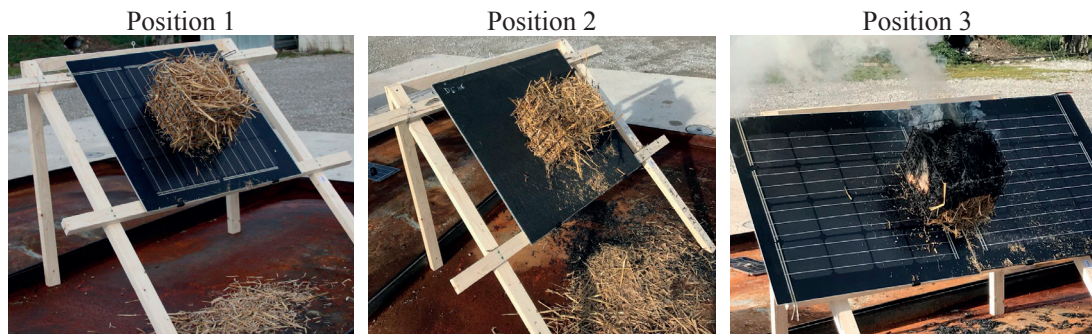
Figure 8.4 – The test setup to evaluate the fire resistance include a wood support, a lightweight module and a basket with brands, in accordance with CEN/TS 1187 (Method 1).
