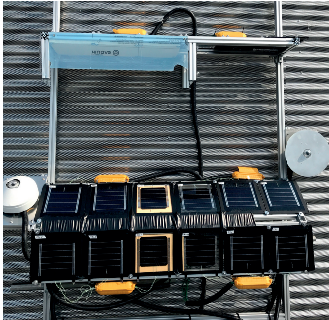
Figure 8.8 – Mock-up installation for monitoring the cell and module operating temperature. Three different module designs are analyzed: glass-glass configuration, PO/Al-based and PO/aramid-based lightweight module. This installation simulates two different types of integration: a well-ventilate installation and a non-ventilated installation.
